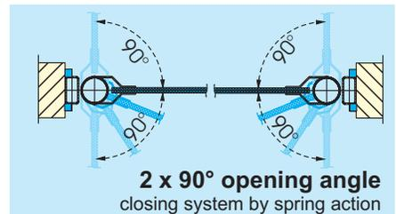
**Swing door panels PTK 35** highly transparent or combined with blue, red and black. Thickness 5, 7 and 10 mm. Excellent transparency, highly abrasion resistant, age- and UV-resistant, high breaking strength in coldness, standard quality up to -30°C, low-temperature proof up to -45°C.
